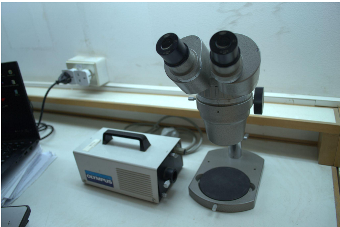
a. Photo of the CBRL, OLYMPUS SZ-III/SZ-Tr - Zoom-Stereo microscope set-up
